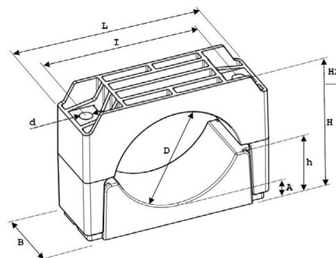
Initial torque for fastening fixing material : 5 – 8 Nm.
